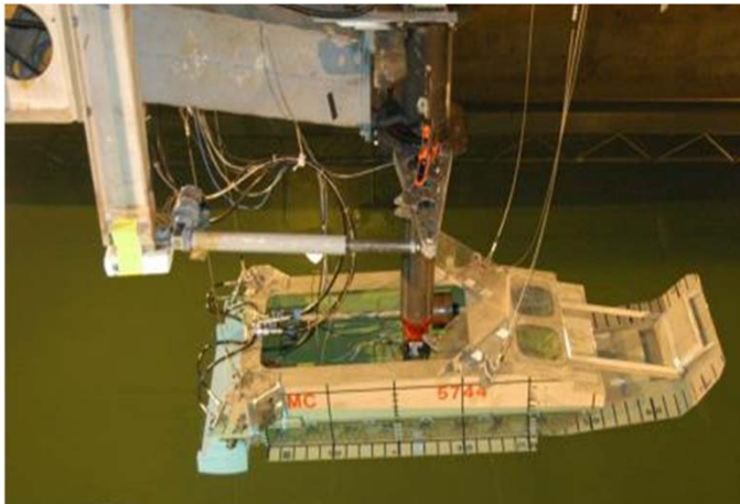
Model Testing – Extended Bow & Aft Lifting Body
