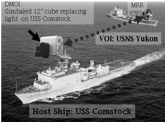
Figure 4: DMOI installed on the O7 level of the USS Comstock–LSD45 (host vessel) used to interrogate the MRR on the VOI.
