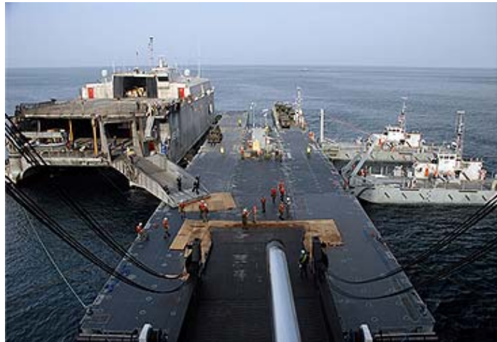
Figure 5-2: RRDF Operations as viewed from Sealift Ship Stern with connector on the left and tugs on the right
