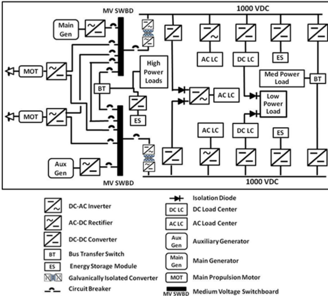
Figure 1. Notional Naval Ship Electrical Architecture (MVDC Ring Bus)
