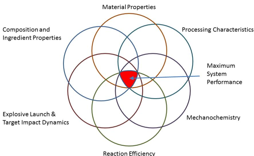
FIGURE 2. TYPICAL FACTORS WHICH INFLUENCE COMBUSTION EFFICIENCY IN METAL/METAL COMPOSITE MATERIALS
