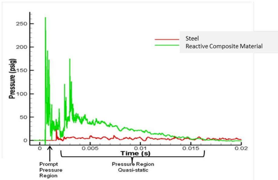
FIGURE 1. TYPICAL PLOT OF THE ENERGY RELEASE IN A COMBUSTION CHAMBER COMPARED TO THE ENERGY RELEASE OF A STEEL FRAGMENT OF THE SAME MASS
