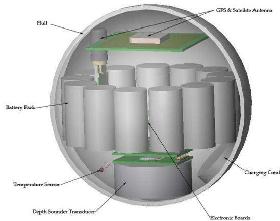
*Figure 1. Cross-Sectional Schematic View of Riverine Drifter.*
