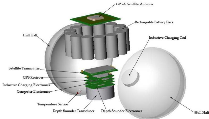
*Figure 2. Exploded Schematic View of Riverine Drifter.*
