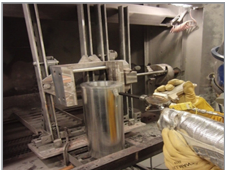
Innovative cold spray repair technology for ships. Courtesy of iMAST.
