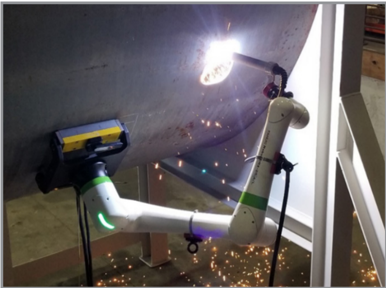
Streamlining Hull Access Welding and Cutting with Automation. (Courtesy of CNM)
