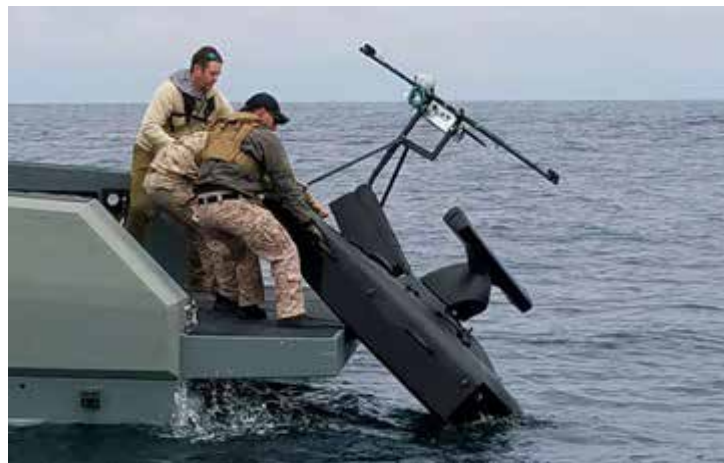
Marines recover the Hydronalix Reckless unmanned surface vessel (USV) after conducting a mission during the ONR GLOBAL-sponsored TOEE 24.1 at Camp Pendleton, California on June 3-14, 2024. (Photo courtesy of ONR GLOBAL)
