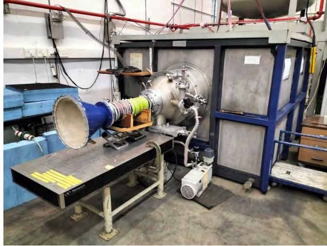
Fig. 17. The 300 kV pulse generator with the magnetron attached to it.
