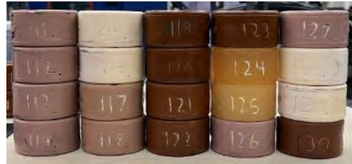
Figure 11. Lineup of some samples fabricated this year, including Alumina (124-125), BST (115-116, 128-129), CCTO (119-123, 130), and CTO (111-114, 117-118, 126-127) composite samples.
