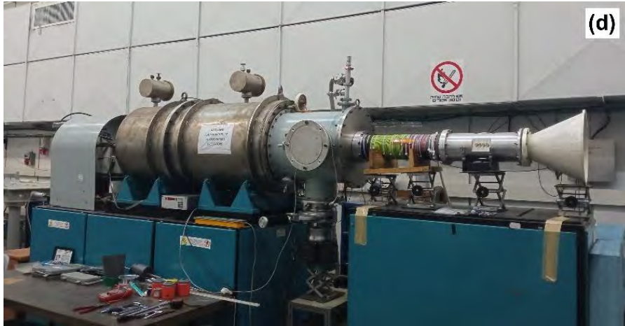
Fig. 11. The LIA - Linear Induction Accelerator with the 3-segment axial output RM attached at its front end.
