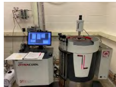
Figure 14. VSM system to measure BH curves.
