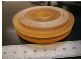
*Additively manufactured high-breakdown-voltage flange designed for high-power microwave (HPM) applications, fabricated using nanocomposite materials with enhanced dielectric strength and dimensional precision.*
