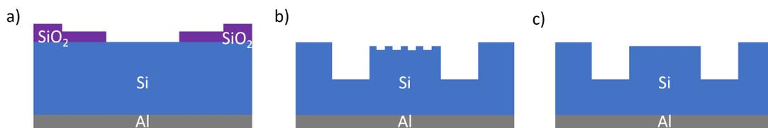
Figure 3: a) Oxide Offset VHELAC cathode. b) Micropillar on mesa VHELAC cathode. c) Mesa VHELAC cathode
