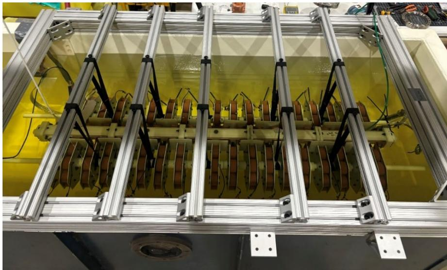
Figure 3: Top-down view of the 19-stage PFN Marx generator hanging from the suspension rack into the oil tank for experimental testing.
