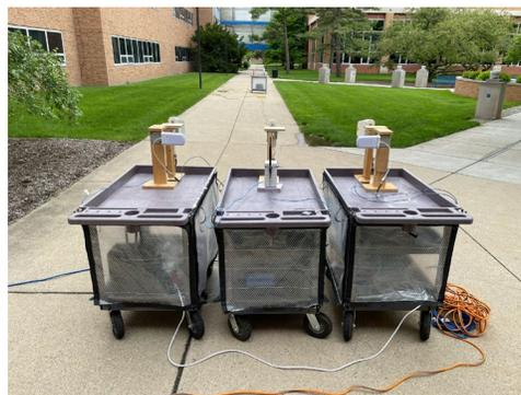
**Figure 6. Photograph of the distributed phased array. Antenna masts are placed along the far edge of the carts.**
