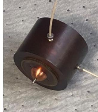
**Figure 37 The Donald was made in house for testing flat and “belly button” electrode profiles.**
