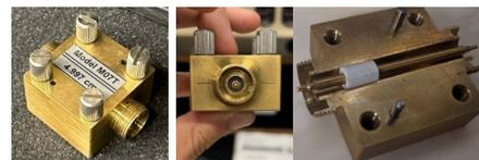
**Figure 1.** MuEpsIn coaxial airline dielectric test fixture (top-left). Test fixture assembled with sample showing a good fit between inner and outer conductor (top-right). Bottom half of test fixture with permittivity sample and inner conductor in place (bottom).
