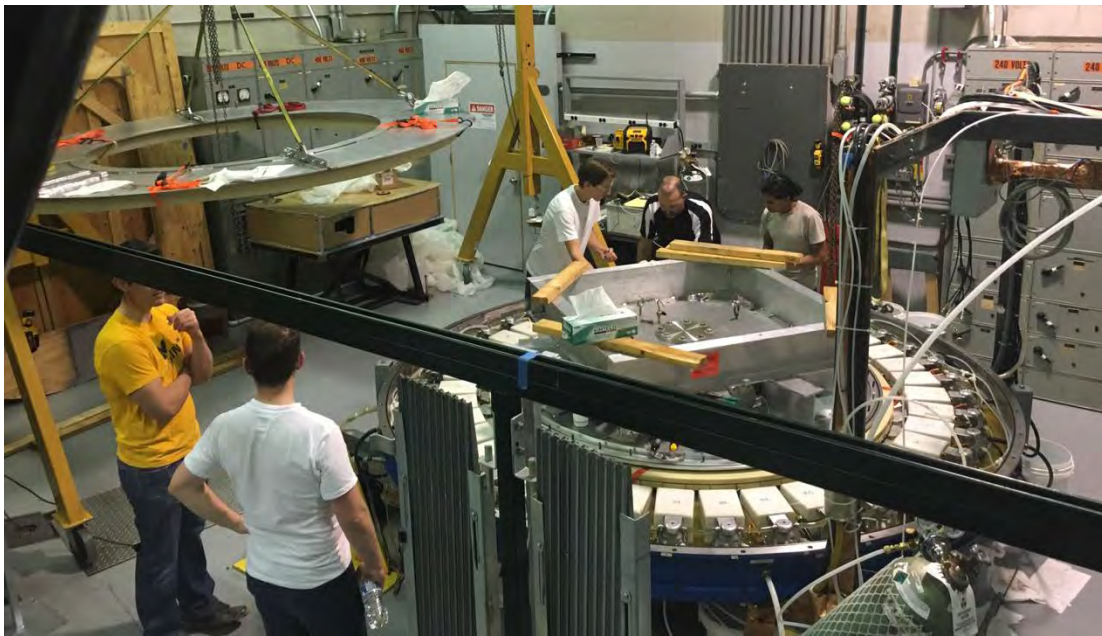
Figure 24. PI Ryan McBride (front left) and Sandian Jon Douglass (front right) as well as Co-I Nick Jordan (back left), Sandian Tommy Mulville (back center), and applied physics PhD student Akash Shah (back right) working on the MAIZE LTD cavity. The L3 switches for BLUE are presently being tested in MAIZE. Significant improvements to UM's LTD facilities were made during this visit.
