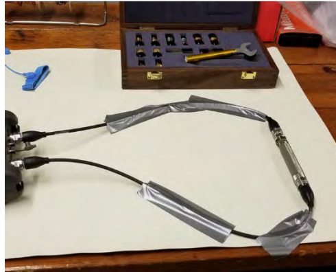
Fig 4 Experimental test setup for dielectric measurements
