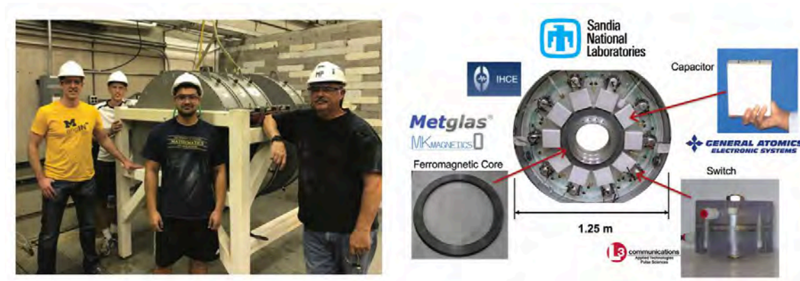
Figure 22. The BLUE pulsed power facility being received at the University of Michigan. These four LTD cavities were previously part of the 21-cavity Ursa Minor facility at Sandia National Laboratories. This technology transfer is part of Sandia's Stevenson-Wylder Gift Program. [Pictured from left to right: Prof. Ryan McBride (PI), Dr. Nick Jordan (lab manager, research scientist, and Co-I), Steven Exelby (HPM PhD student of Prof. Gilgenbach), and Mark Perreault (senior lab technician and safety coordinator)].
