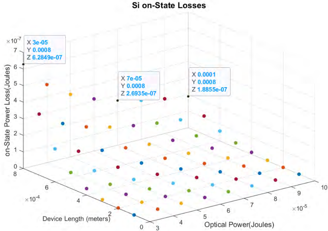
Figure 9: Si on-state losses as a function of path length and optical power. GaN and SiC losses were calculated, but omitted from this report.
