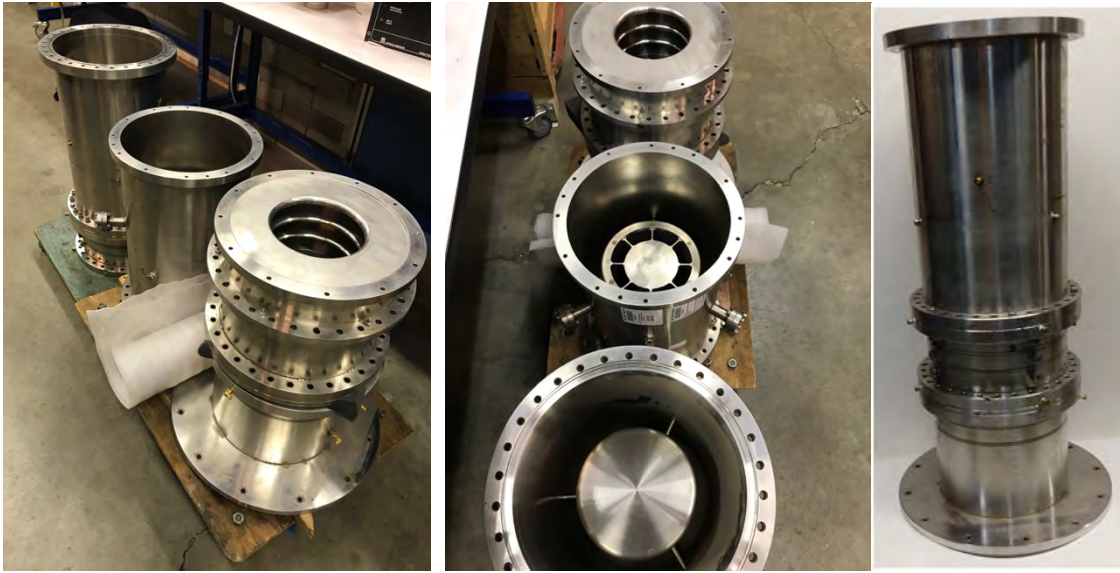
Figure 27. (Left two images) The two brazed MILOs acquired for testing on BLUE. (Right image) The assembled MILO ready to be mounted on BLUE.
