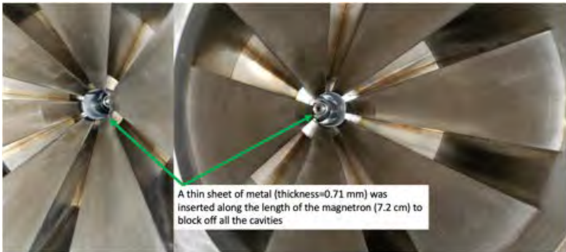
Figure 4. Shim stock was installed to short-out the MDO cavities to observe whether HPRF was being generated by the VC in a vircator-like manner.
