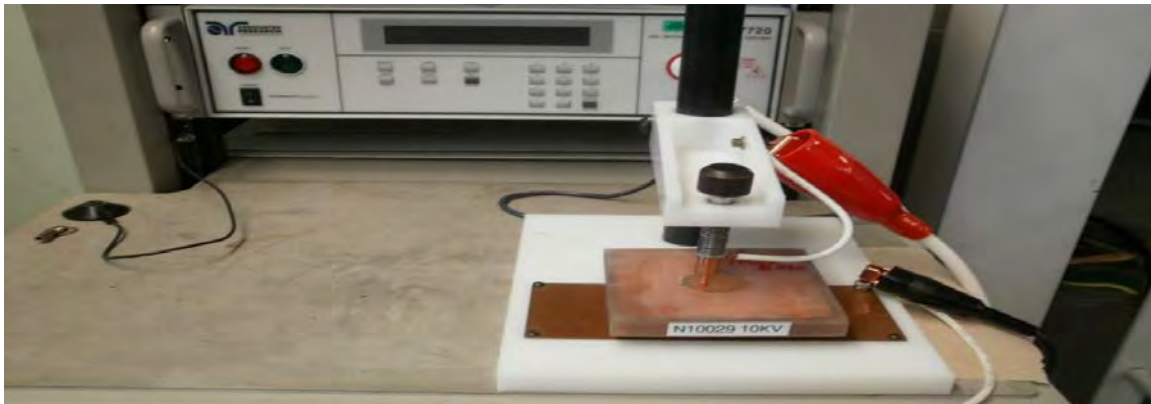
Figure 39: High Potential Test Setup
