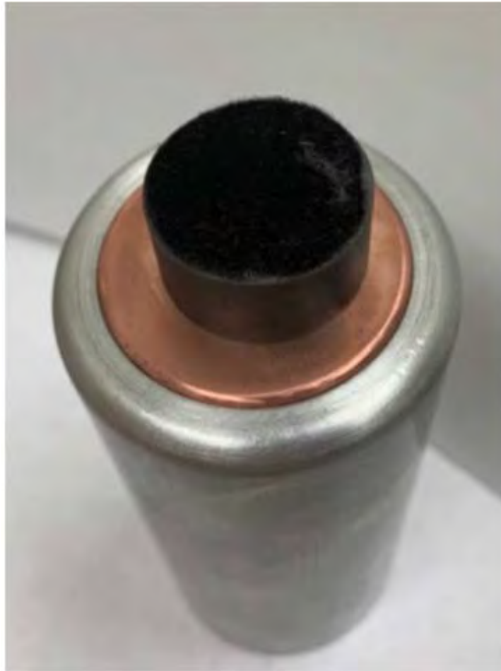
Figure 11. Photograph of cathode prior to mounting on the test bed holder.
