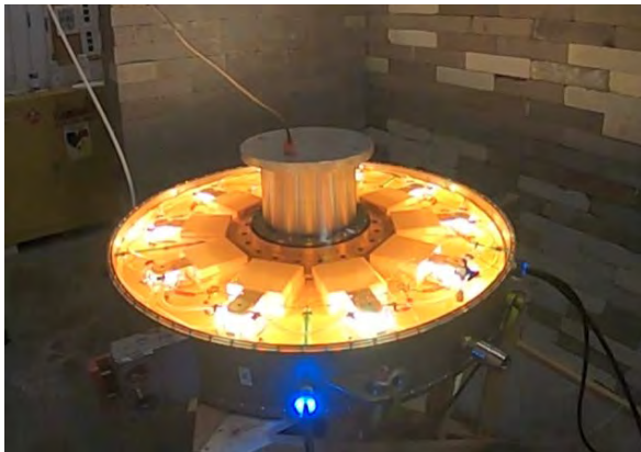
Figure 24. (Left) First shot on BLUE, which was into a resistive load for testing. The clear plastic lid allows the interior of the cavity to be observed during operation and for operation without ferromagnetic cores. (Right) Subsequent pulsed-power testing on BLUE. These are the first 12 shots taken with the newly acquired CVR for current calibration. These shots were taken with charging voltages of +/- 50 kV or +/- 60 kV.
