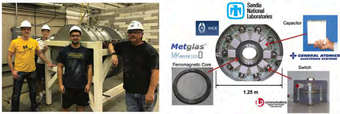
Figure 23. The BLUE pulsed power facility being received at the University of Michigan. These four LTD cavities were previously part of the 21-cavity Ursa Minor facility at Sandia National Laboratories. This technology transfer is part of Sandia's Stevenson-Wylder Gift Program. [Pictured from left to right: Prof. Ryan McBride (PI), Dr. Nick Jordan (lab manager, research scientist, and Co-I), Steven Exelby (HPM PhD graduate of Prof. Gilgenbach), and Mark Perreault (senior lab technician and safety coordinator).]
