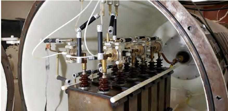
**Figure 2. Photograph of the PI-110A accelerator used for MDO experiments showing solid state resistors replacing liquid resistors (photographed July 13, 2020).**
