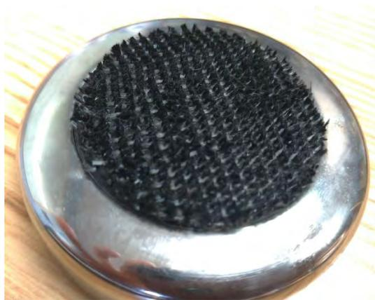
*Figure 20. TTU carbon fiber velvet small cathode*
