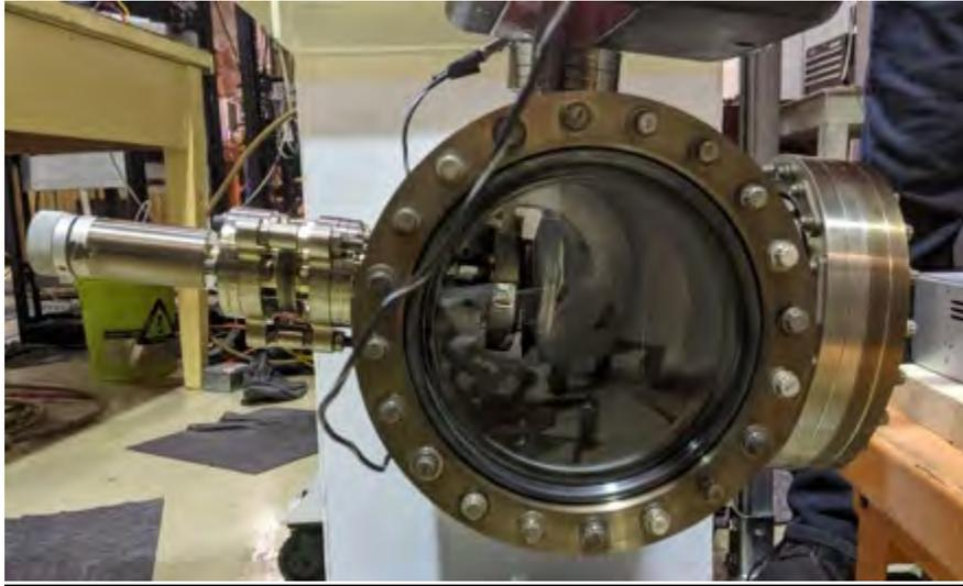
Figure 21. Cathode testing chamber.
