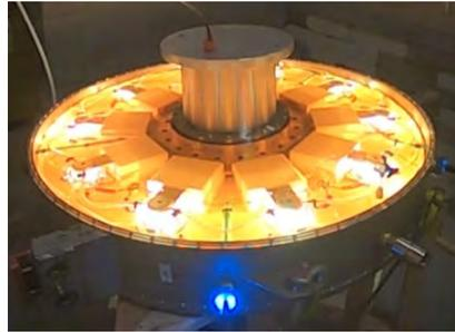
Figure 29. First shot on BLUE. The clear plastic lid allows the interior of the cavity to be observed during operation and for operation without ferromagnetic cores. The resistive load is mounted within the vacuum chamber on top of the cavity.
