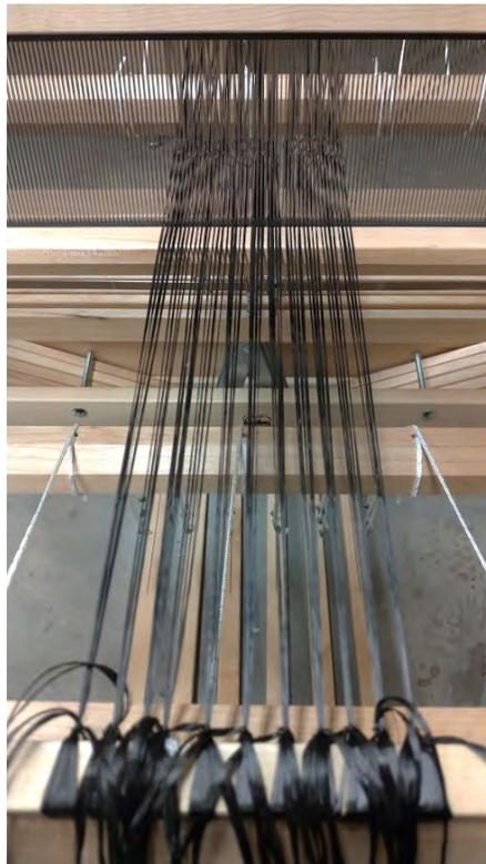
*Figure 18. Carbon fiber thread mounted on the loom.*
