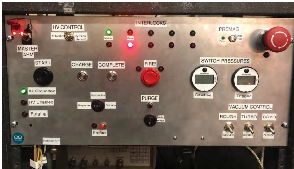
Figure 48: Arduino Uno (ATmega328P-based) control panel for semi-autonomous control of the BLUE charging and firing sequence, as well as other system functions.
