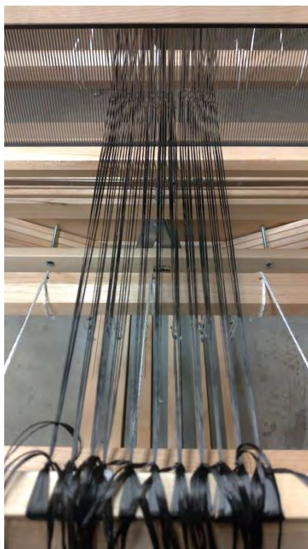
Figure 34. Carbon fiber thread mounted on the loom.
