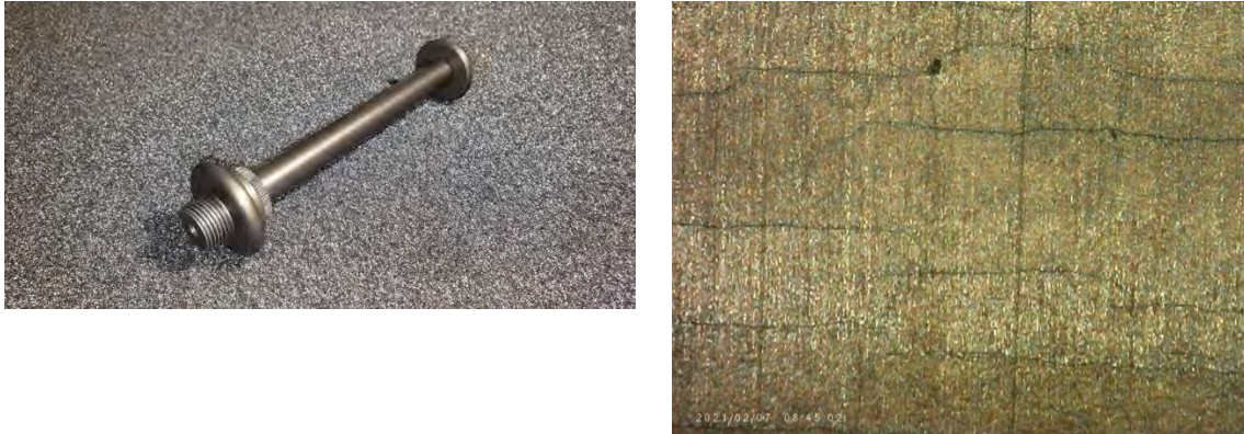
Figure 5. Left: Photograph of the anodized split cathode parts that were shipped to NSWC. Right: Photograph of the anodization taken through a microscope.
