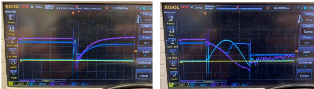
Figure 12. Sample scope data measured during a discharge (left) and recharge (right). Notice how the voltage waveforms (purple and dark blue) do not match the expected results from simulations above at all.
