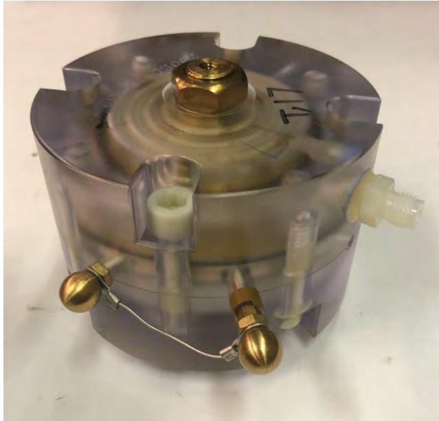
Figure 47: An L3Harris spark-gap switch with brass electrodes, capable of operation at 200 kV ( \pm 100 kV) and up to 200 psi gas fill. These switches are used in the MAIZE and BLUE LTD systems at the University of Michigan. In this image, the switch is shown with a shorting wire between the UV-pin and mid-plane. In the BLUE cavity, the shorting wires are replaced with 3-M \Omega resistor chains for proper operation of the UV-pin.
