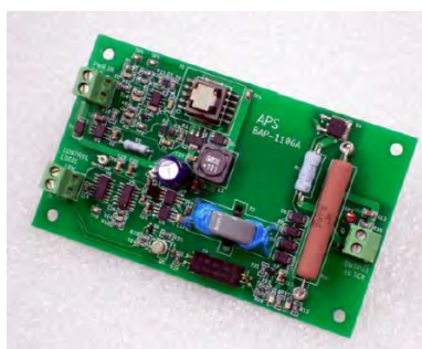
Figure 10. APS SCR trigger boards we bought to replace our custom-made ones.
