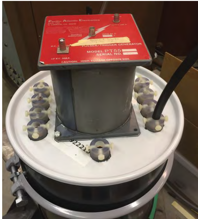
Figure 50: The 10-gallon oil drum containing the trigger pulse generating brick, which is charged in parallel with the BLUE LTD cavities and triggered by the PT55 pulse generator mounted to the top of the drum.
