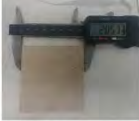
Figure 1. As sintered ceramic pieces of Barium Strontium Titanate (~2.9 inches square)
