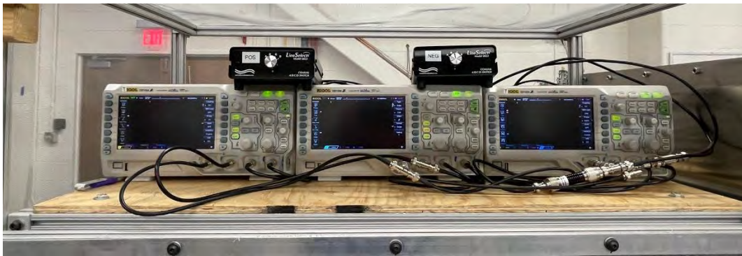
Figure 17. One to four BNC splitter boxes installed on the testbed.
