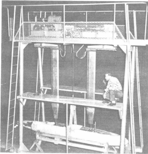
Fig. 7. Tilt table with model attached mounted on storage stand
