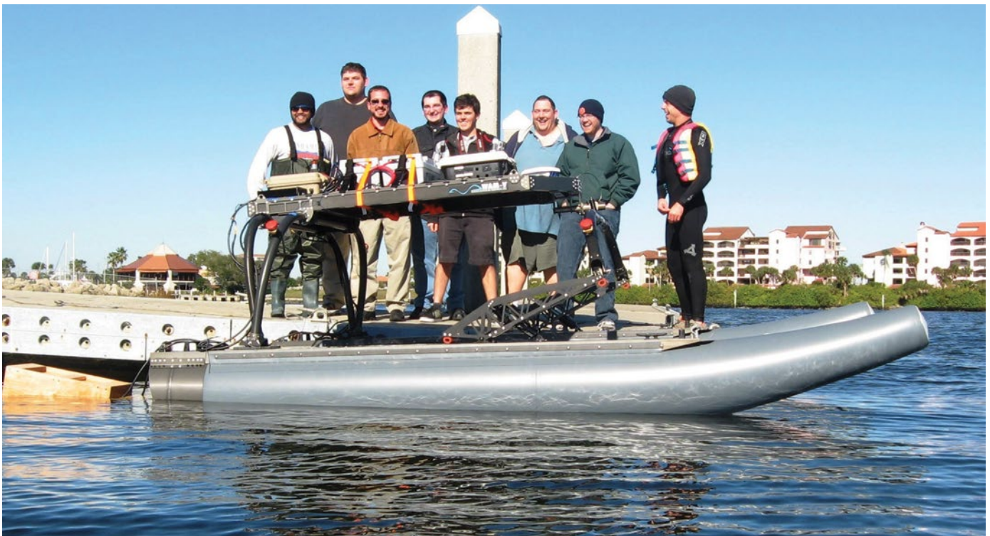
Each team in the Maritime RobotX Challenge will use a standard wave-adaptable modular vehicle (above) that they will then modify with their own electric propulsion system. Embry-Riddle Aeronautical University (opposite) is one of 15 teams competing in the event (Photos courtesy of AUVSI Foundation)
