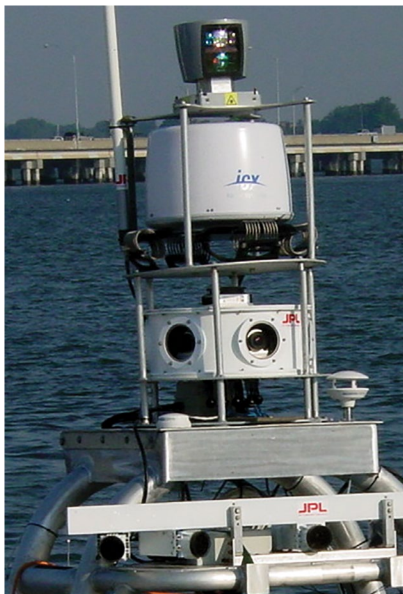
Pictured here is the sensor suite for the Control Architecture for Robotic Agent Command and Sensing (CARACaS) autonomous control system. From bottom to top: stereo electro-optic, 360-degree electro-optic, radar, and lidar. (Photo from Naval Surface Warfare Center).
