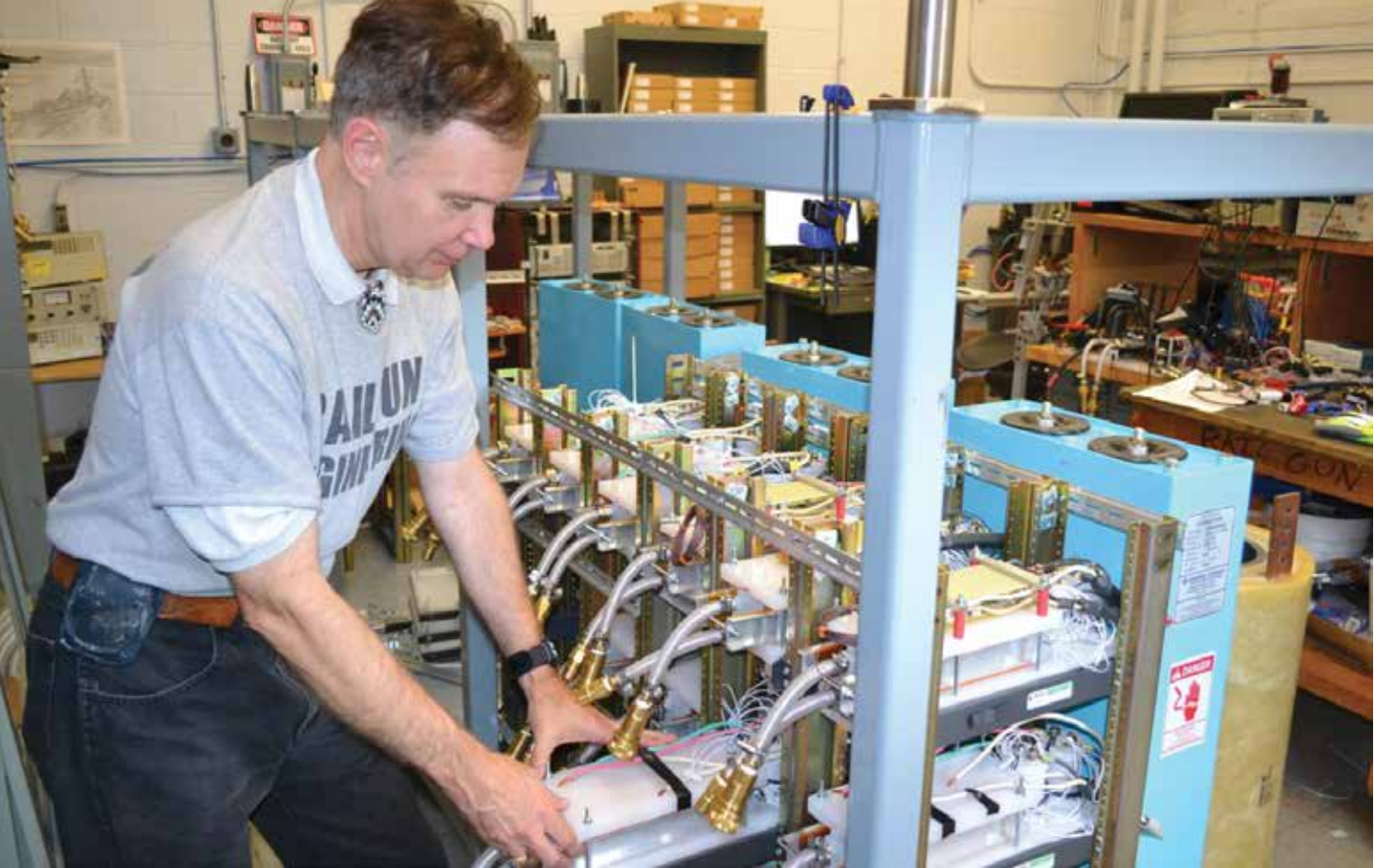
A research engineer installs a pulsed power battery pack at NRL. The Pulsed Power Physics Branch is developing a scaled facility to evaluate battery-based pulsed power systems. The battery packs will charge the capacitor over several seconds, which when triggered will release 60 kilojoules of stored energy into the inductor and resistive load in milliseconds.
