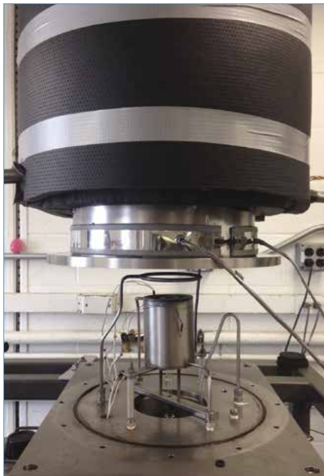
Metal halide co-condensation reactor built and operated by Johns Hopkins University, University of Maryland, and Indian Head. Inside the furnace (lower center), molten aluminum is reacted with hydrogen halide gas to produce metastable aluminum monohalide vapors that are condensed on the stainless steel bell jar.
