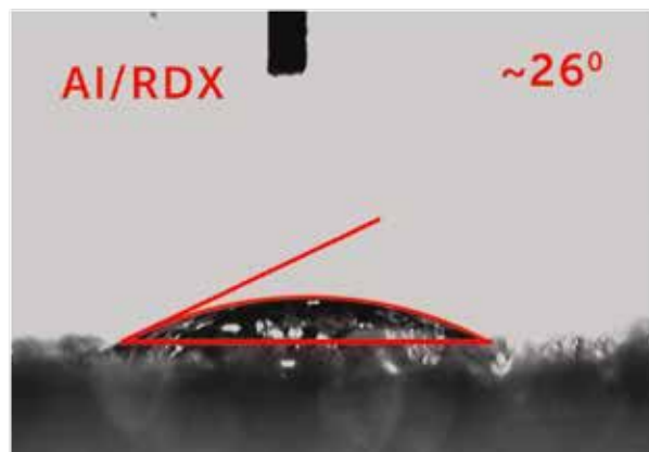
H 2 O contact angle analysis of particles of bare RDX and RDX-coated with about 900 nm of aluminum.
