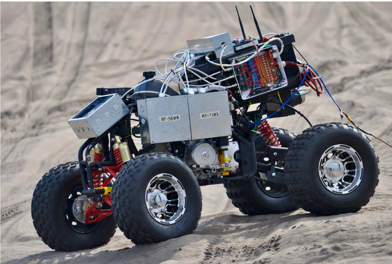
Currently being tested on an autonomous land vehicle in Chile, the Polar TRACER algorithm is designed to help unmanned vehicles navigate in featureless environments such as Antarctica. (Photo by ONR Global)
