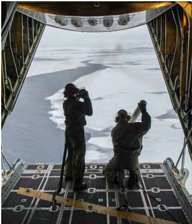
Crew members aboard a Coast Guard C-130 launch expendable current probes while on a flight over the Arctic during an Office of Naval Research-sponsored expedition to study the seasonal ice zone. (Photo by John F. Williams)
