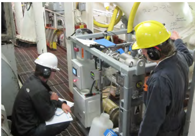
Naval Research Laboratory researchers collect a ballast water sample aboard M/V Indiana Harbor. They are using the shipboard filter skid to collect organisms by concentrating them in miniature plankton nets contained within the oblong silver housings (the housing visible in the photo is marked "A").
