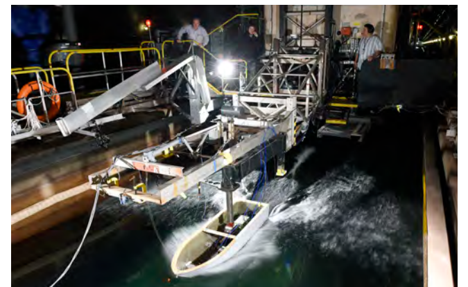
A ship hull model attached to a high-speed carriage moves through waves at the Naval Surface Warfare Center Carderock Division's David Taylor Model Basin. The project's purpose is to study the fundamental physics of the water impact of high-speed planing hulls and to measure the slamming loads and resulting motions of the craft upon re-entry into the water. (Photo by John F. Williams)
