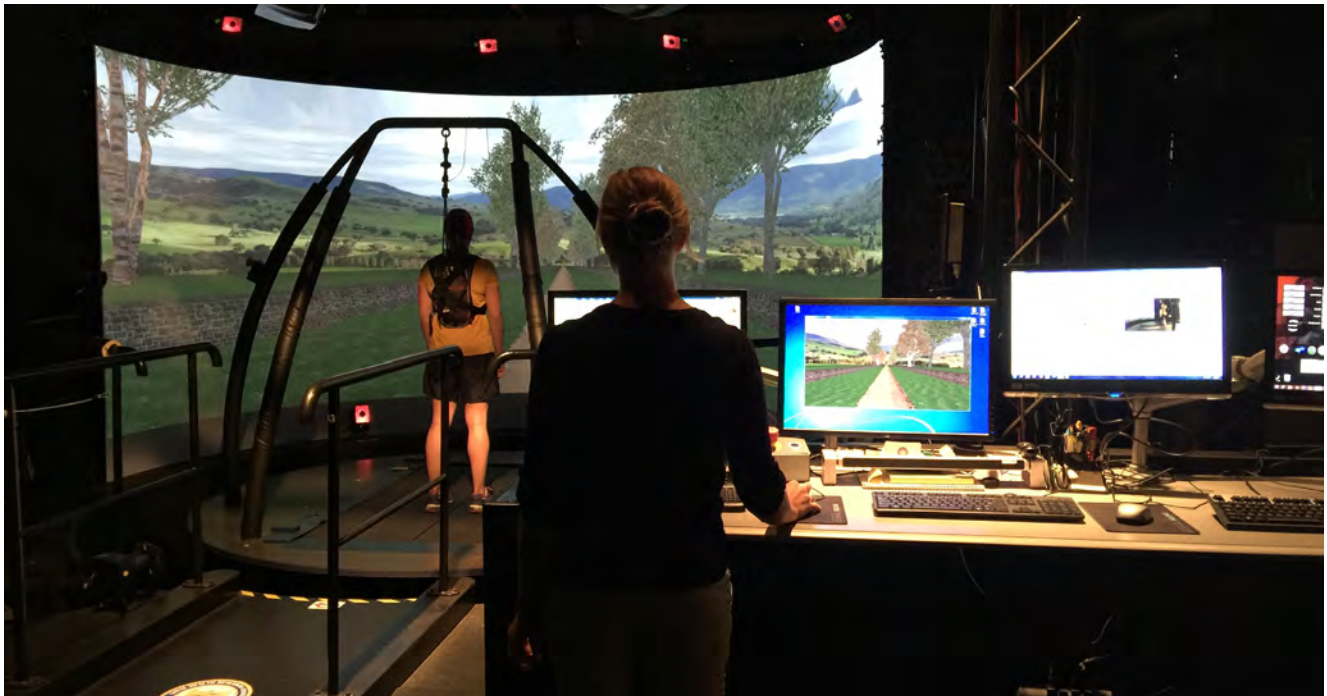
The Naval Health Research Center conducts research using the Computer Assisted Rehabilitation Environment (CAREN), an immersive virtual reality system. The CAREN is made up of a 9-foot diameter platform with integrated treadmill and 180-degree wide, 9-foot tall curved projection screen. The CAREN is used for studies related to survivability, equipment loads, rehabilitation, and fatigue. Photo by Regena Kowitz
