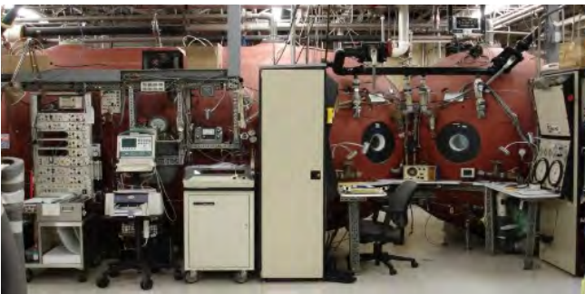
The hyper/hypobaric chamber and associated measurement equipment.
