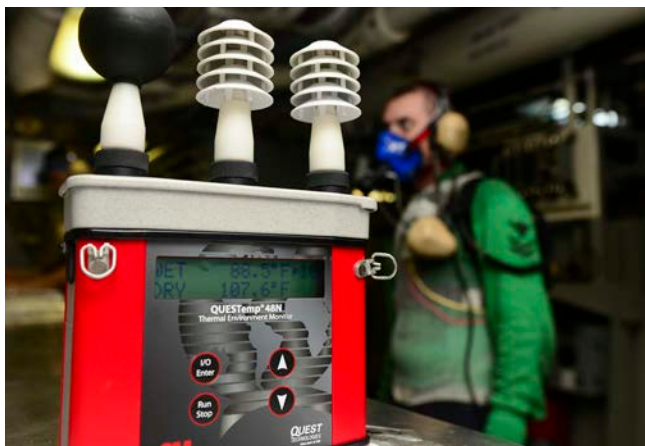
To gather data about environment conditions in work spaces aboard Nimitz, Naval Health Research Center personnel used a thermal environment monitor that measures both the wet and dry temperatures. Photo by MCSN Jose Madrigal
