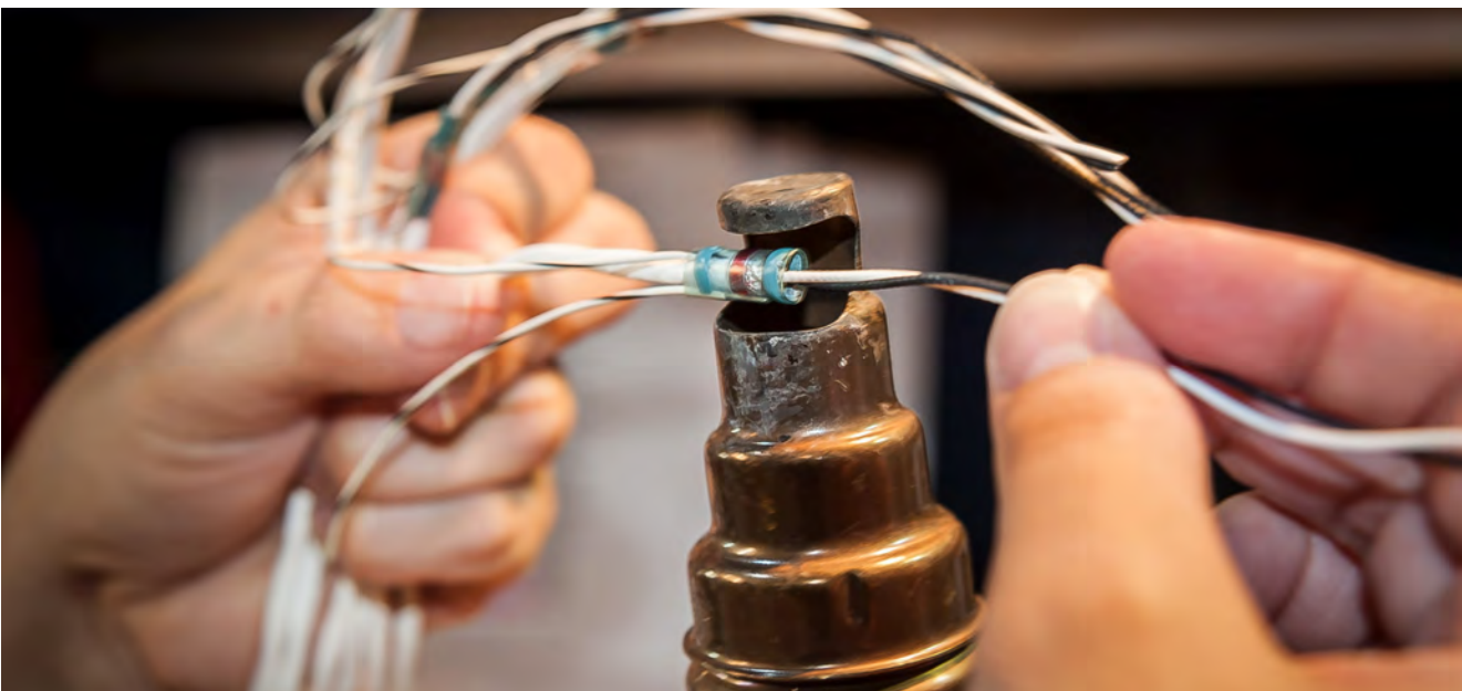
SSC Atlantic contract personnel from an 8(a) small business manufacture cables for the Mine Resistant Ambush Protected (MRAP)/ All-Terrain Vehicle program. Photo by Joe Bullinger
