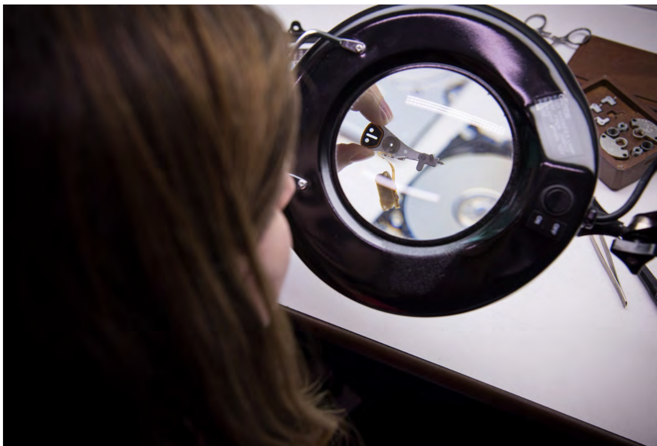
SSC Atlantic employee Alisha Slebodnik performs an examination of the head stack from a computer hard drive on a "clean bench." Slebodnik works in the Digital Media Criminal Forensics Investigations Laboratory. Photo by Joe Bullinger
