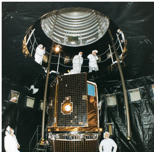
This is a final look at the Clementine DSPSE spacecraft, which is mated to its launch vehicle, the Titan IIG (two i's, not two ones). Here, the nose fairing is being lowered to enclose Clementine in its new home during launch.
