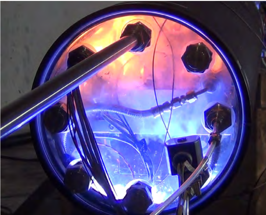
An experiment validates the applicability of water for a lithium-ion battery casualty suppression system. Unmanned underwater vehicles do not typically use see-through bulkheads and endcaps, but during this experiment polycarbonate end-caps were used on the test article to allow direct imaging of behaviors in the battery vessel during casualty initiation, fire progression, fire-suppression, and resolution of the test event at Naval Surface Warfare Center Carderock Division. Photo by NSWC Carderock Division Imaging Branch
