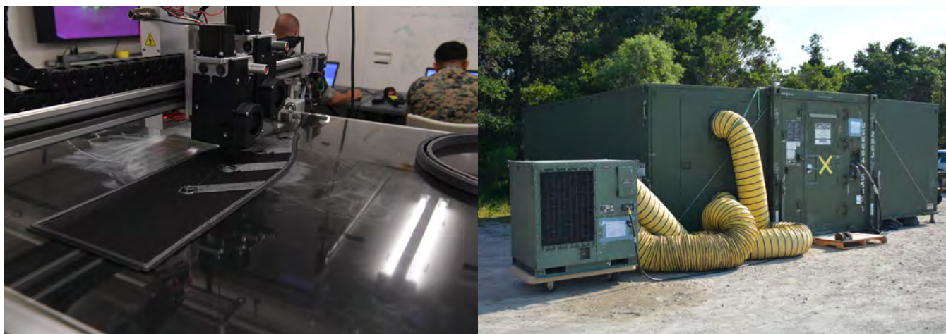
A 3D platform Work Series 300 (left) prints a shell for a boat mold as part of the Advanced Naval Technology Exercise East at Camp Lejeune, North Carolina. Naval Surface Warfare Center Carderock Division's Advanced Manufacturing Project Office demonstrated the use of the expeditionary fabrication facility, which used a 20-foot expandable shipping container (right) as a printing lab in the field. Photos by Kelley Stirling and Edward Adamos
