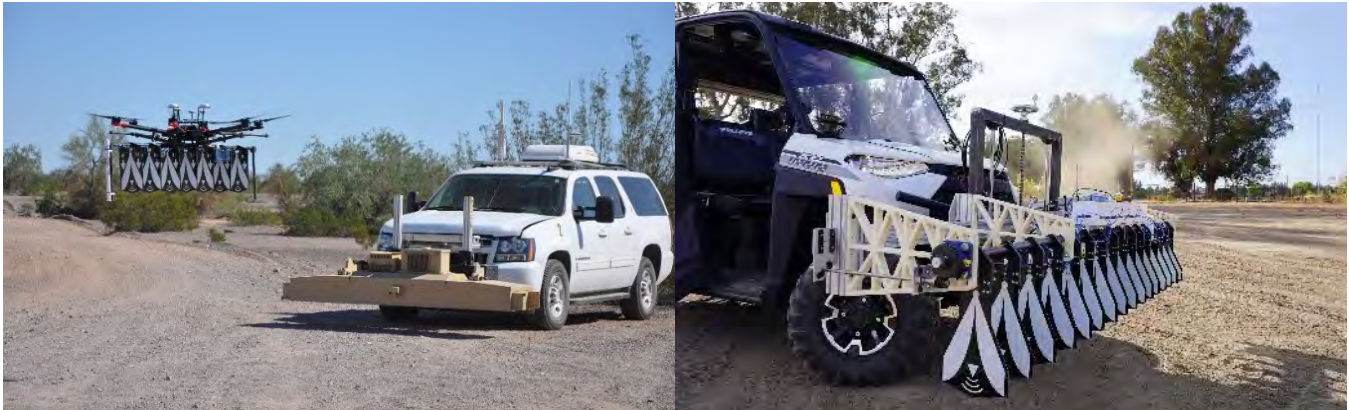
On the left, field trials with first unmanned aerial multistatic ground penetrating radar system flies in front of a vehicle-mounted prototype array. On the right, a new miniaturized-scalable 16-channel system on a Polaris vehicle is shown prior to its first field test.
