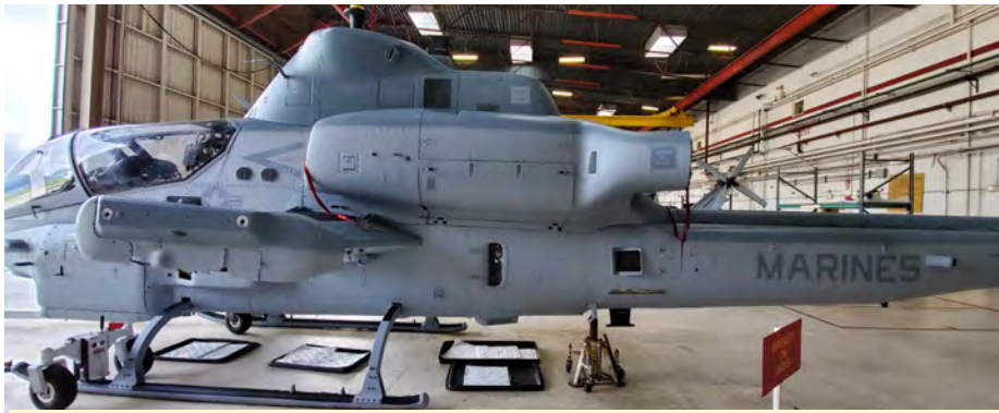
A Marine Corps AH-1Z Viper helicopter is painted with a camouflage gray polysiloxane topcoat, which was developed by chemists at the Naval Research Laboratory for aircraft to be safer for the environment and easier to apply. Photo by Erick Iezzi
