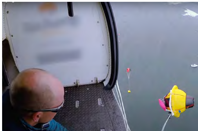
At about 12 pounds, Spotter buoys are light enough to be deployed from either ships or aircraft and allowed to drift with ocean currents. Photo provided by Sofar Ocean
