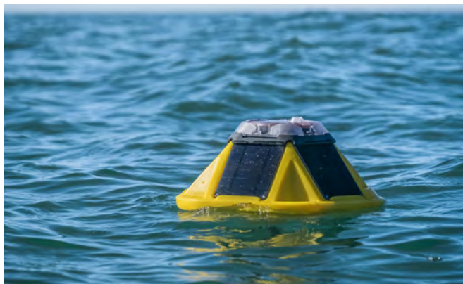
Solar-powered Spotter buoys can be moored in a single location for long-duration data collection. Photo provided by Sofar Ocean
