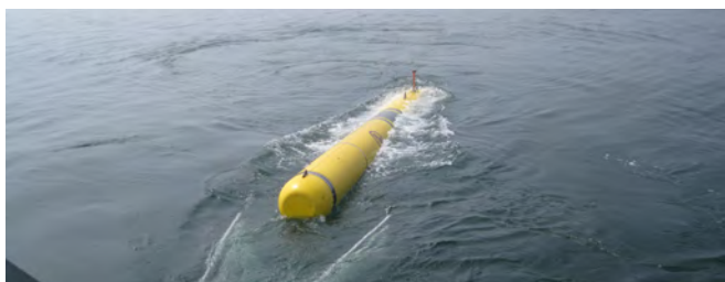
The NRL Acoustic Division's Black Pearl autonomous underwater vehicle being recovered in the approaches Boston Harbor carrying advanced structural acoustics sonar payloads. Black Pearl is an updated vehicle with a second-generation sonar carrying with it the ability to do low-frequency broadband (LFBB) at much longer ranges. LFBB is an active sonar that employs synthetic aperture processing and the processing also uses artificial intelligence to detect and classify objects of interest. Photo by US Naval Research Laboratory
