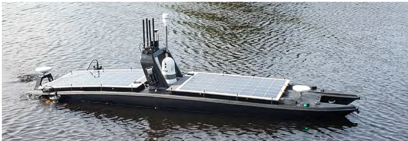
A close up of the 12-foot MANTAS vehicle shows its various instruments and solar panels. Photo by Maritime Tactical Systems, Inc
