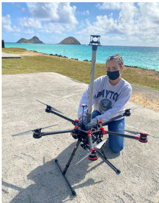
Melissa Sanders, a mechanical engineer at Naval Information Warfare Center Indo-Pacific Department, tests a DJI S900 hexacopter with a Tri-Sonica Mini-Weather Sensor at Bellows Air Force Station in Hawaii. Photo by Dexter Barit
