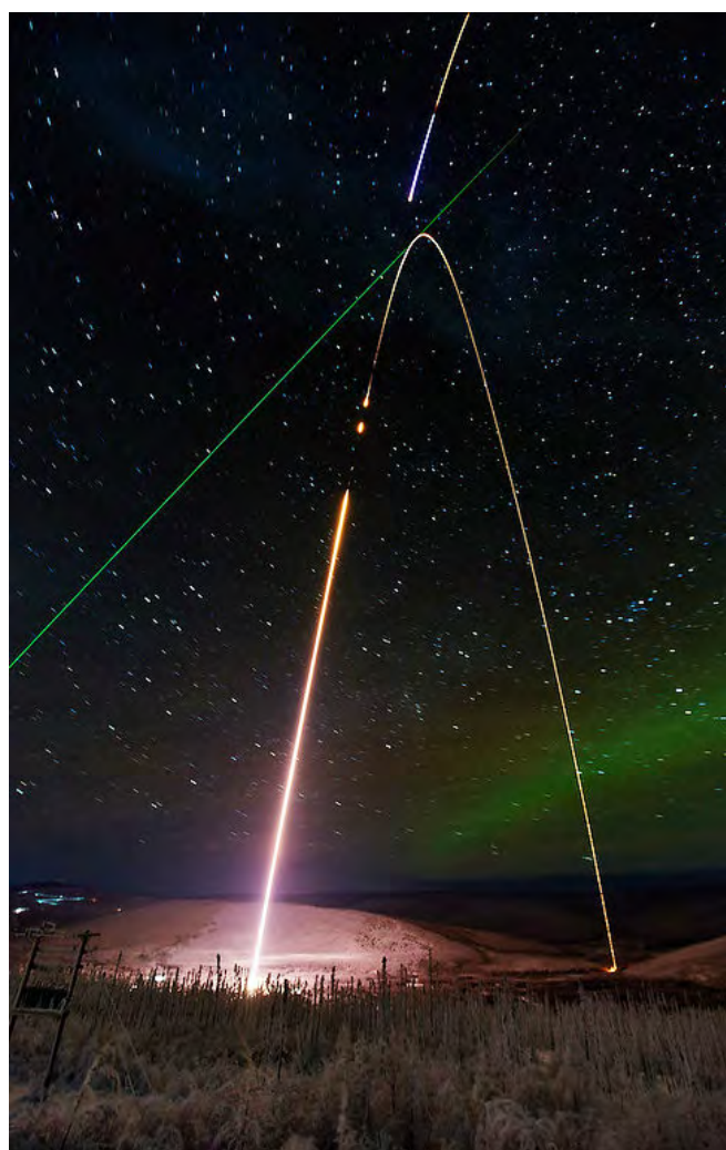
A long-exposure view of the NASA "Super Soaker" rocket trail to its destination altitude of 53 miles, along with the lidar beam (green) used for temperature measurements and cloud detection. The launch was part of a NASA and US Naval Research Laboratory study showing water vapor, a common launch byproduct of space traffic, can actively cool the mesosphere and induce the formation of mesospheric clouds. Photo by NASA Wallops Flight Facility
