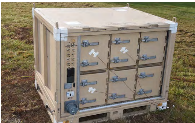
Naval Surface Warfare Center Carderock Division's Charging-capable Li-ion Autonomous Safe Storage Interservice Container (CLASSIC) before being tested during a battery burn demonstration at the Aberdeen Proving Ground in Maryland. Photo by Thomas Hays
