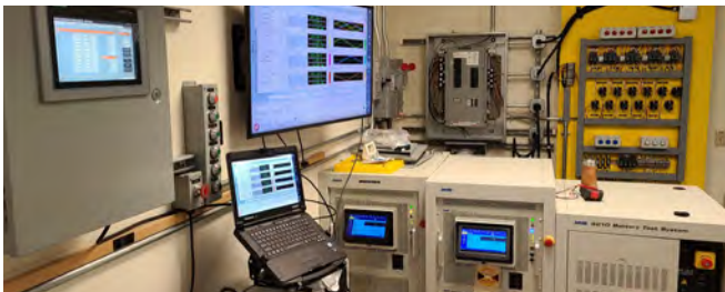
The Energy Innovation Laboratory's full-scale power grid simulator testbed supporting development of advanced sub-metering to optimize energy, water, and wastewater with data.
