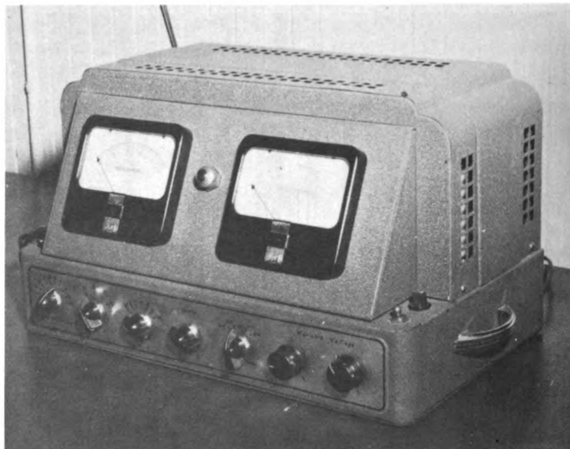
Figure 8. Portable polarograph designed and assembled at the University of Oregon by Dr. Paul Delahay.
