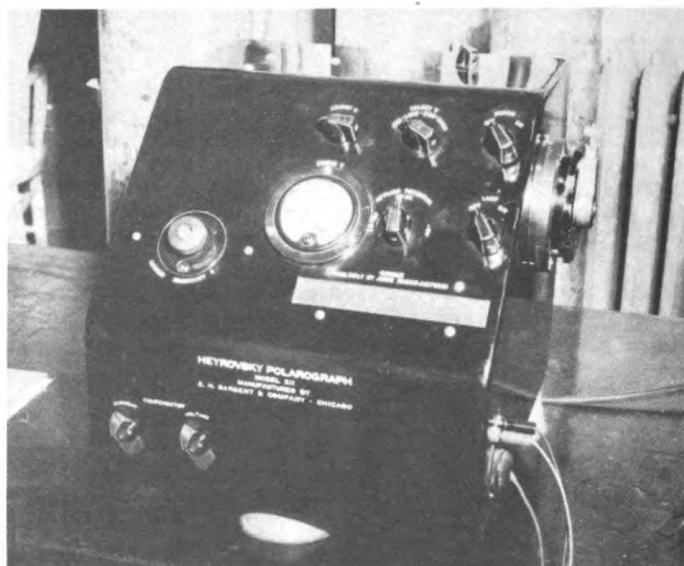
Figure 9. Sargent Polarograph of the Heyrovsky type with automatic photographic recording of current-voltage curves.
