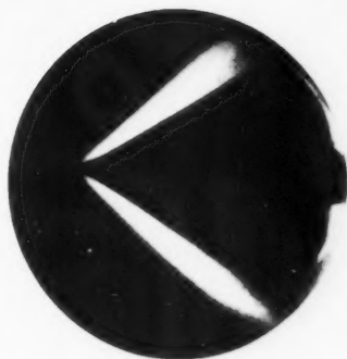
Figure 10 - Luminous flow of xenon over a model wedge viewed through window of tube.
