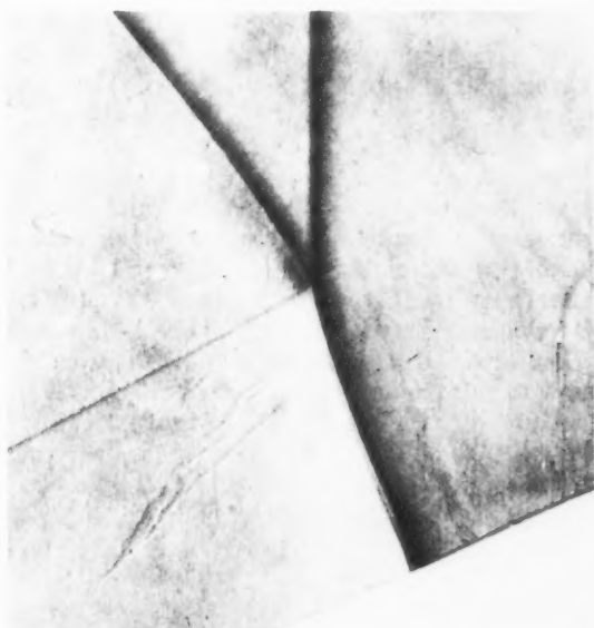
Figure 9 - Reflection of a shock wave from the surface of a wedge.
