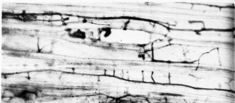
A section of yellow pine infected by a marine fungus. The infected areas appear as dark lines
