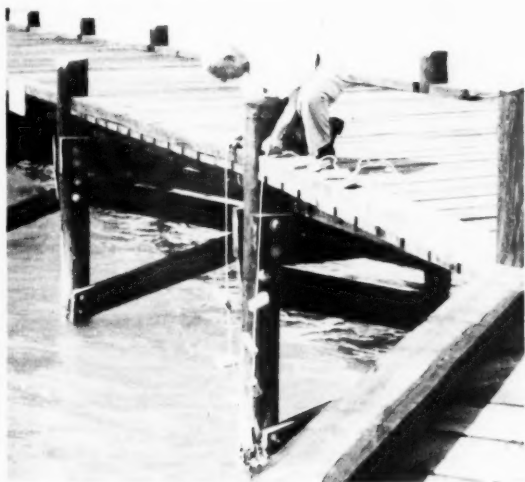
Dr. E. S. Reynolds exposes wood panels to sea water at the Marine Laboratory pier.
