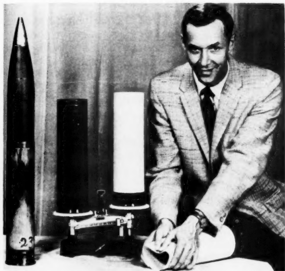
Stanley P. Prosen, NOL scientist, displays sample plastic cartridge case. Present steel case weighs down the scale. On the left is an assembled 105-millimeter artillery shell, the plastic case of which has been test-fired six times at NOL.
