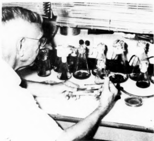
Dr. E. S. Reynolds inoculates flasks with pure cultures of marine fungi. The flasks contain wood in nutrient solution.
