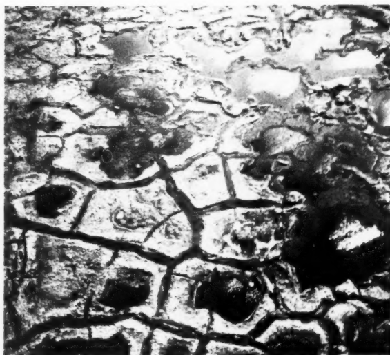
Figure 4 — Oblique aerial view of flat and marginally ridged polygons and of coal-escing thaw ponds. The polygons at lower center are about 10 to 20 feet in diameter.
