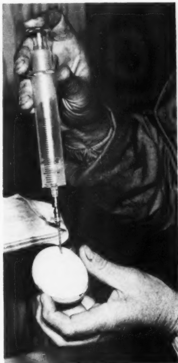
The radio thermometer and empty penguin egg shell are readied for use. Left, the telemeter is placed in shell. Right, albumen is injected into sealed shell.
