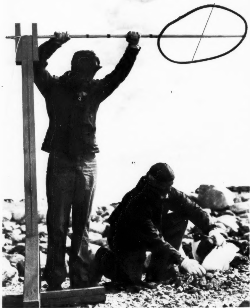
Frederick E. Charlton orients loop antenna over penguin nest as Carl Eklund places egg containing telemeter under bird. Temperature signals picked up by the antenna are carried by a transmission line to a receiver located nearby.
