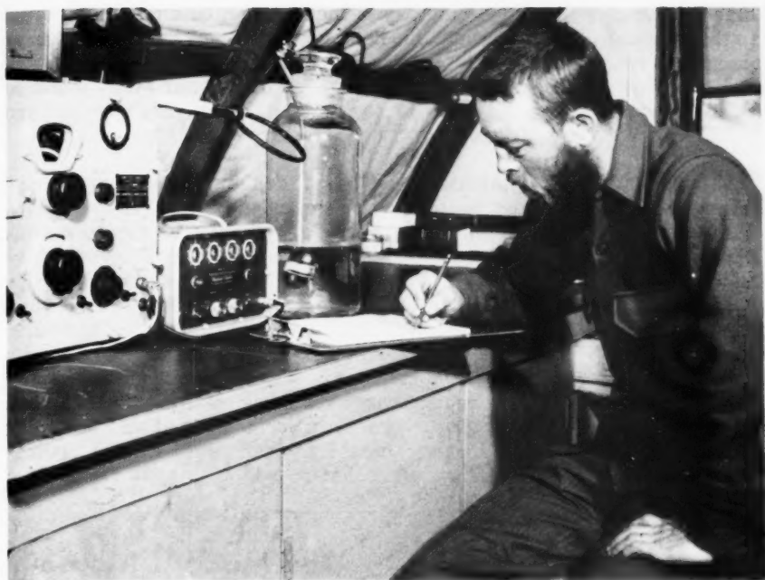
Charlton calibrates temperature telemeter. Instruments shown, from left to right, are receiver, counter, and telemeter (in bottle).
