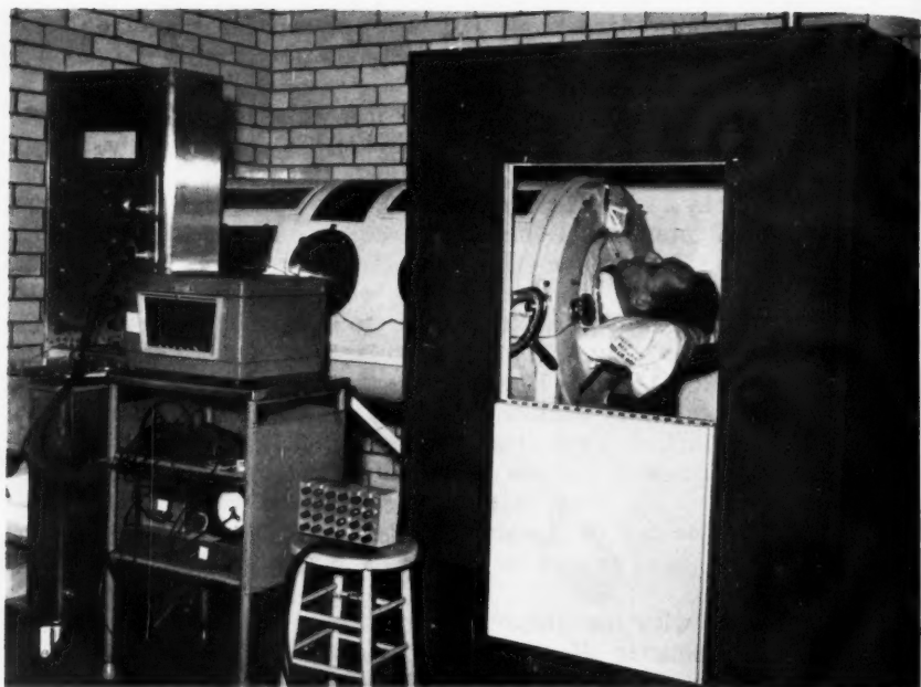
A human volunteer enclosed in tank-type respirator designed to deprive him of the usual input to his senses. The photograph above shows the complete assemblage of equipment, including the screen (at right) and "polygraph" and tape recorder (at left). The photograph below shows the "head" end of the tank; a voice-activated microphone and self-feeding device can be seen mounted on the tank above the subject's head.
