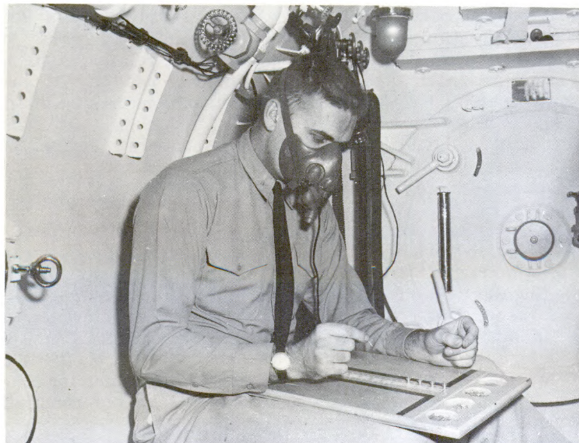
Figure 5--Test for manual dexterity inside the decompression chamber
