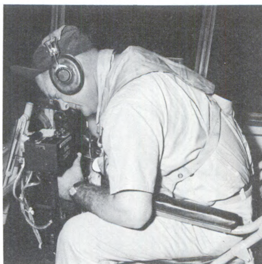
Figure 11-- Operating the drift sight.
