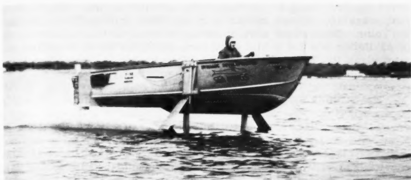
The XCH6 experimental vehicle--built for research purposes, especially to demonstrate the validity of supercavitation principles.
