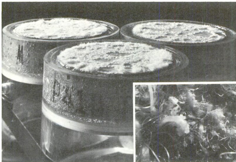
Salt-growth whiskers. Inset: powerful magnification of whiskers.
