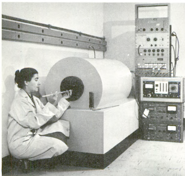
Low-level beta counter radiation shield made from a section of the barrel of an 8-inch gun, as installed for use at Brookhaven.
