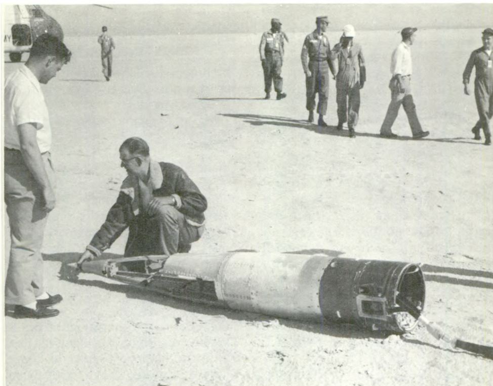
Nose cone of the Aerobee-Hi Rocket after recovery at White Sands, New Mexico. The spectograph containing the "Lyman alpha" profile camera was found elsewhere, having separated from the nose cone.
