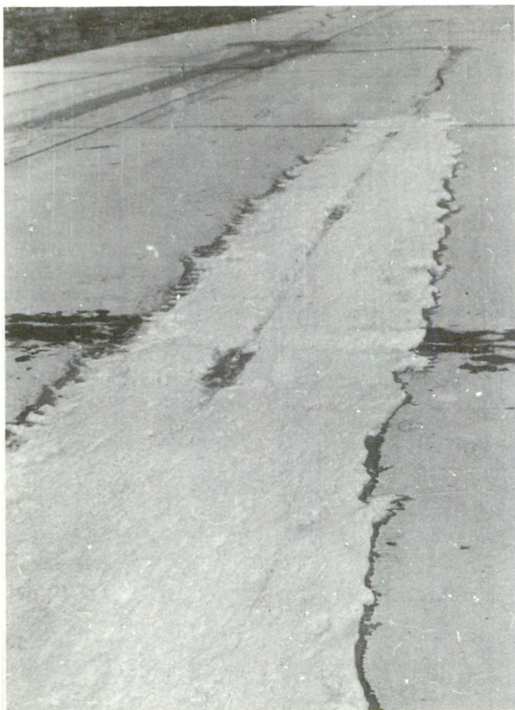
Figure 6--Foam pattern 60 minutes old, illustrating the complete lack of water runoff.
