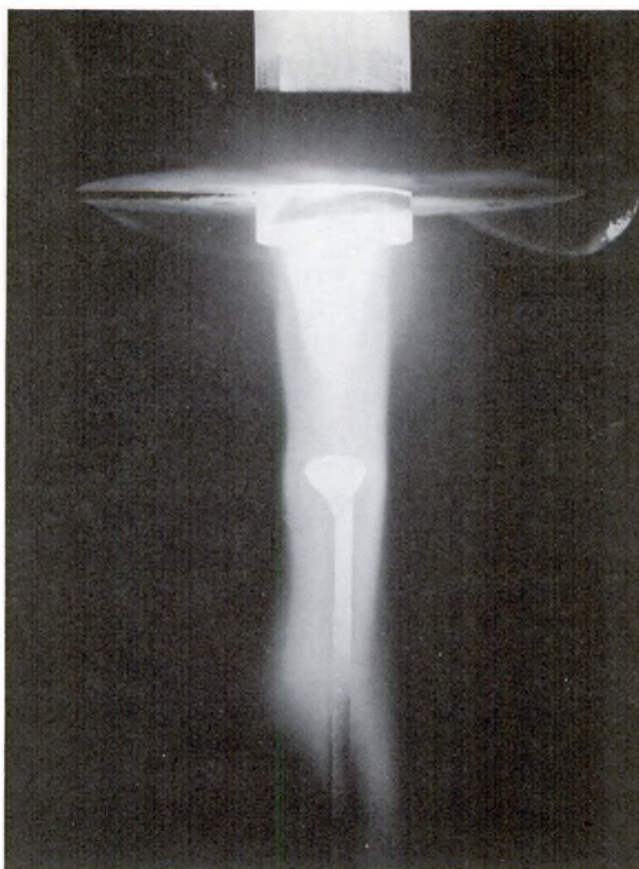
Figure 2--A later model of the torch melts the top end of an aluminum oxide rod to grow an artificial sapphire.
