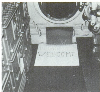
Figure 5 - Latex paint on floor mat. The paint exhibited only slight wear after one month of service. (Photo courtesy of Bu-Ships)
