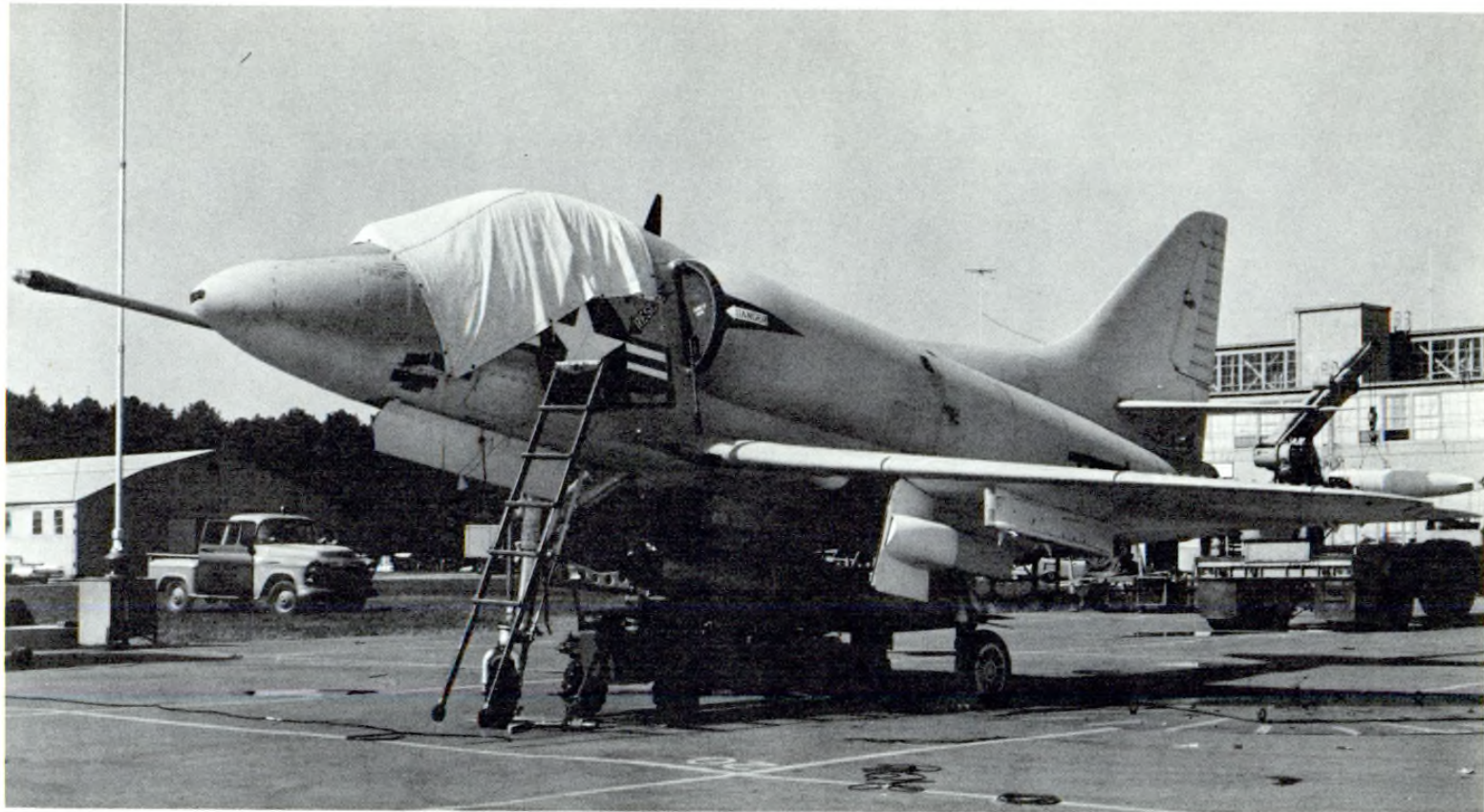
Instrumented aircraft, bomb, and bomb truck on the 360° turntable of a simulated aircraft carrier deck at NWL, Dahlgren. The antenna at the left is used during electromagnetic radiation tests on the bomber's ordnance in connection with Project HERO.
