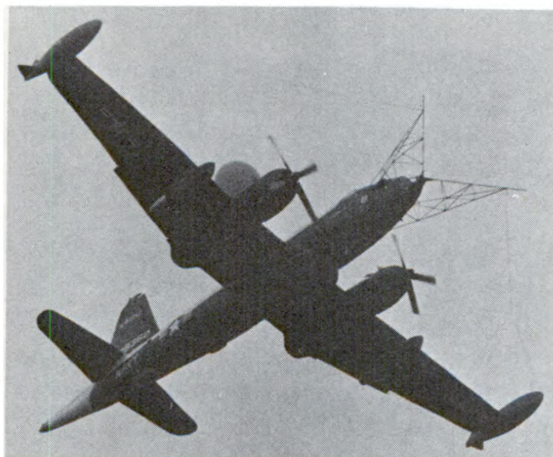
A Navy P2V Neptune equipped with special pickup fork gets ready to "rescue" survivor.
