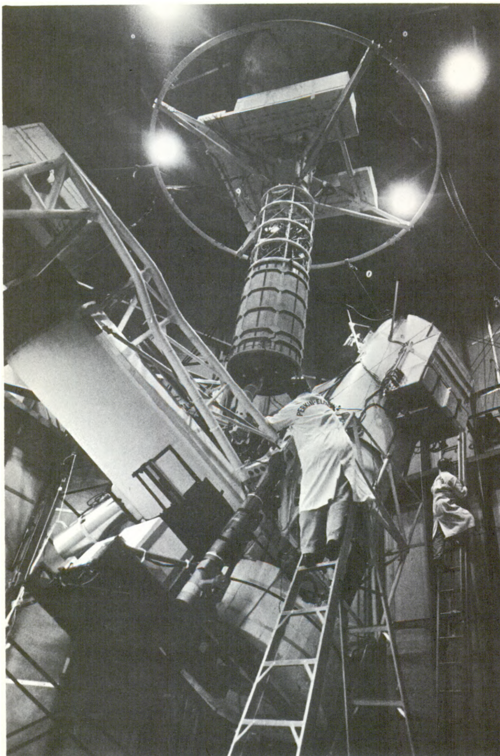
Technicians check out the 6,300-pound Stratoscope II telescope system which early next year will be lofted by balloon to 80,000 feet—above almost all of the Earth's atmosphere—to make infrared observations of Mars. See article beginning on page 7.
