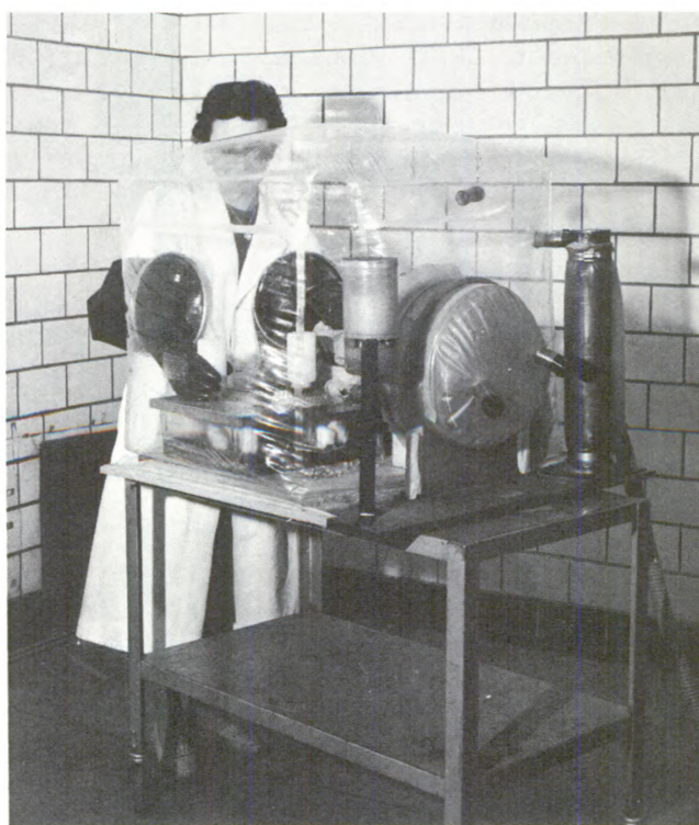
Chemically sterilized plastic isolator. Visibility and flexibility of the plastic greatly facilitates handling of animals by means of sealed-in rubber gloves.
