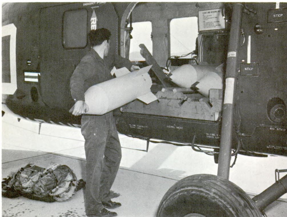
Installing dropsondes in a helicopter prior to release over shot point
