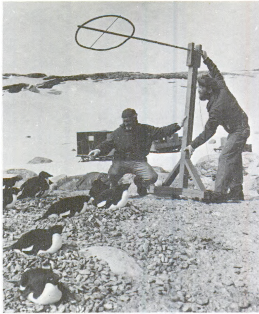
Scientists prepare telemetering equipment and penguin egg for recording incubating egg temperatures remotely.
