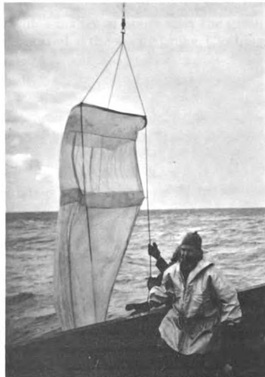
Top, oceanographers retrieve sampling bottles; above left, the Barnes infrared thermometer mounted on bow of M/V OB; above right, a plankton net is lowered.
